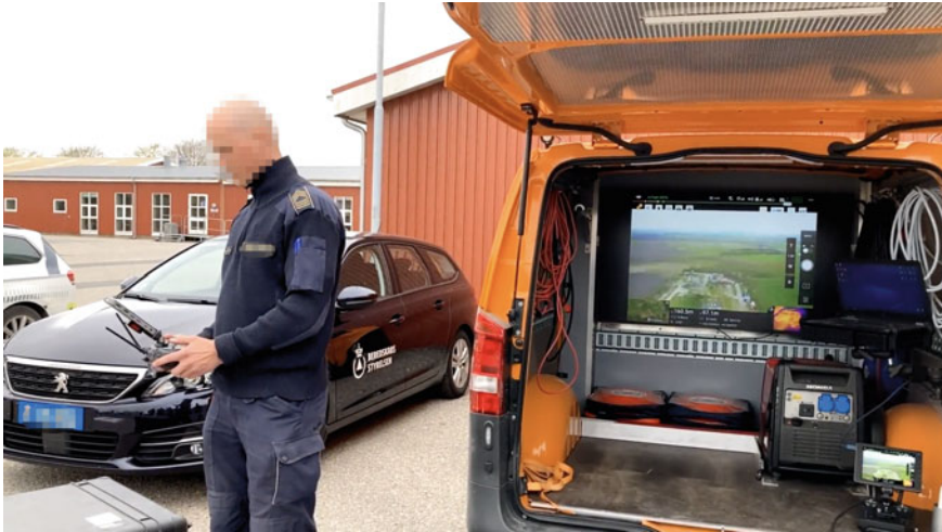
Fig. 11.2 DEMA drone pilot using the DJI smart controller for controlling a single drone, with the video feed shown on the large screen in the support vehicle
